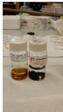
Figure 1.2- Ag-GO solution and Ag-Gr precipitate
